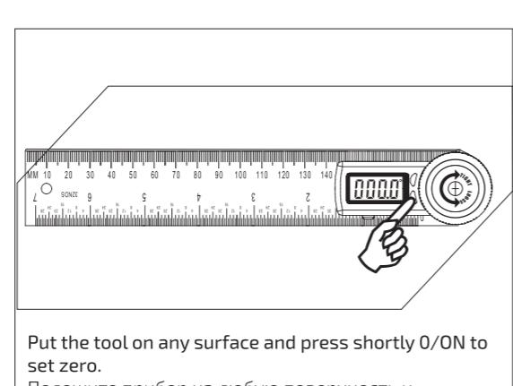
Put the tool on any surface and press shortly 0/ON to set zero.
