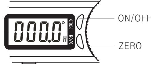
**ON/OFF** Short press ON/OFF to turn on the device. Short press ON/OFF to shut off the LCD. Long press ON/OFF for more than 3 seconds to shut off the whole system. Automatically shut off function in 6 min. Move the scale to turn on the device when at off LCD status.
